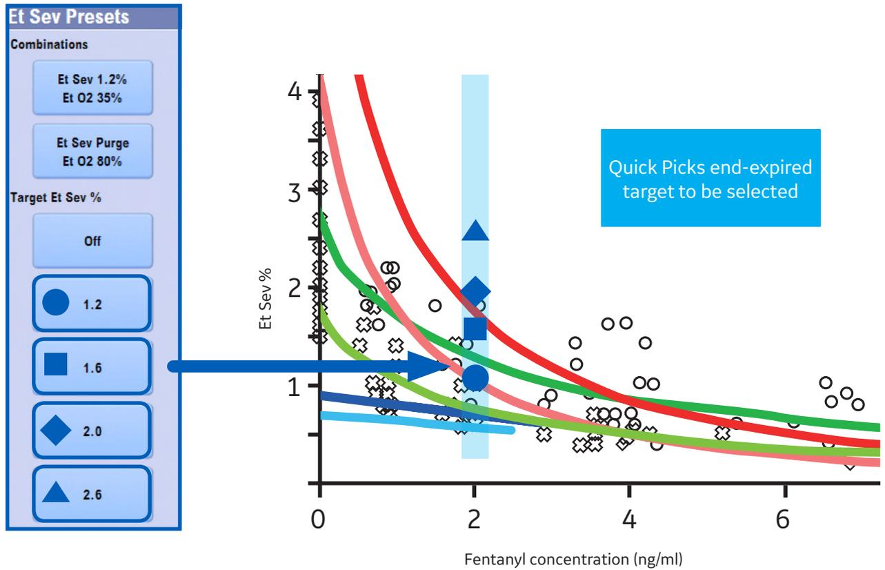
Figure 12: Quick Picks presets and their corresponding locations on Katoh's graph shown here as an example for 2ng/ml fentanyl, O<sub>2</sub>/air
