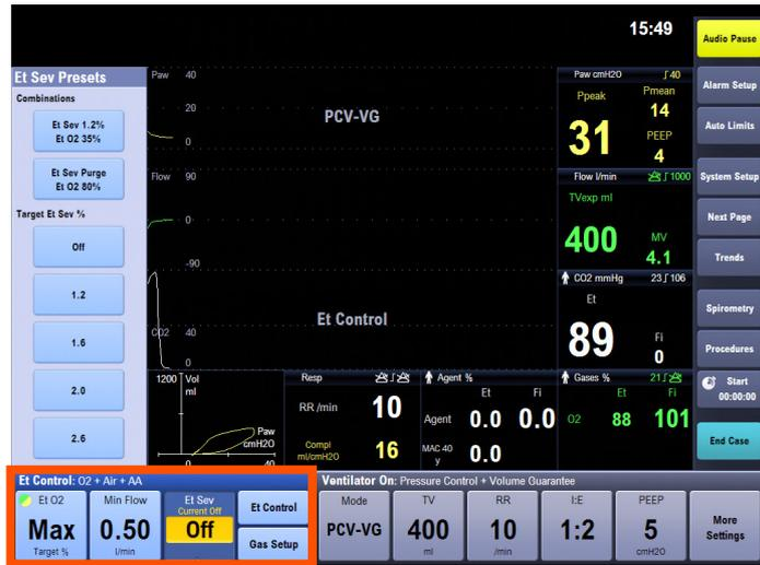
Figure 7: Automated FGF setting mode for end tidal control
