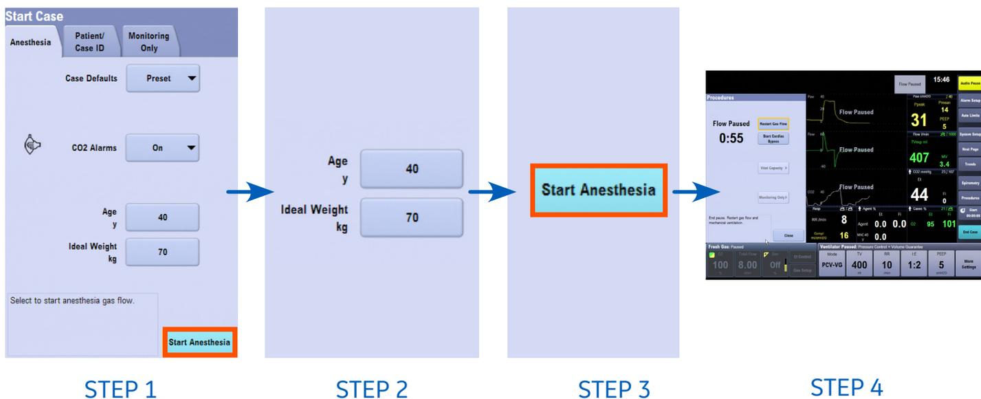
Figure 3: Straightforward steps to induce low flow anaesthesia
