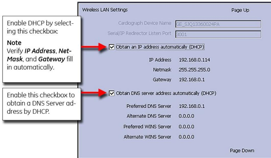
If your network uses static IP addresses, configure the **Wireless LAN Settings** as follows:
