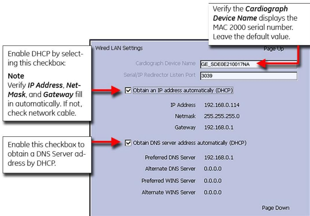
If your network uses static IP addresses, configure the **Network LAN Settings** as follows:
