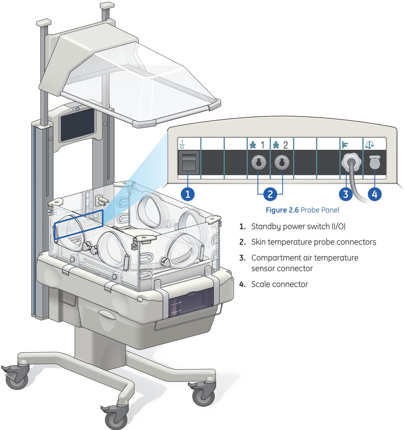
Figure 2.6 Probe Panel
