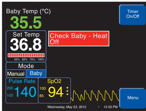
Figure 7.28 Heat Off Alarm Message
