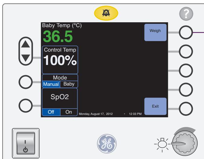
4. You will be prompted to check **Level bed . . .** to ensure that the bed is level during the weighing procedure.
