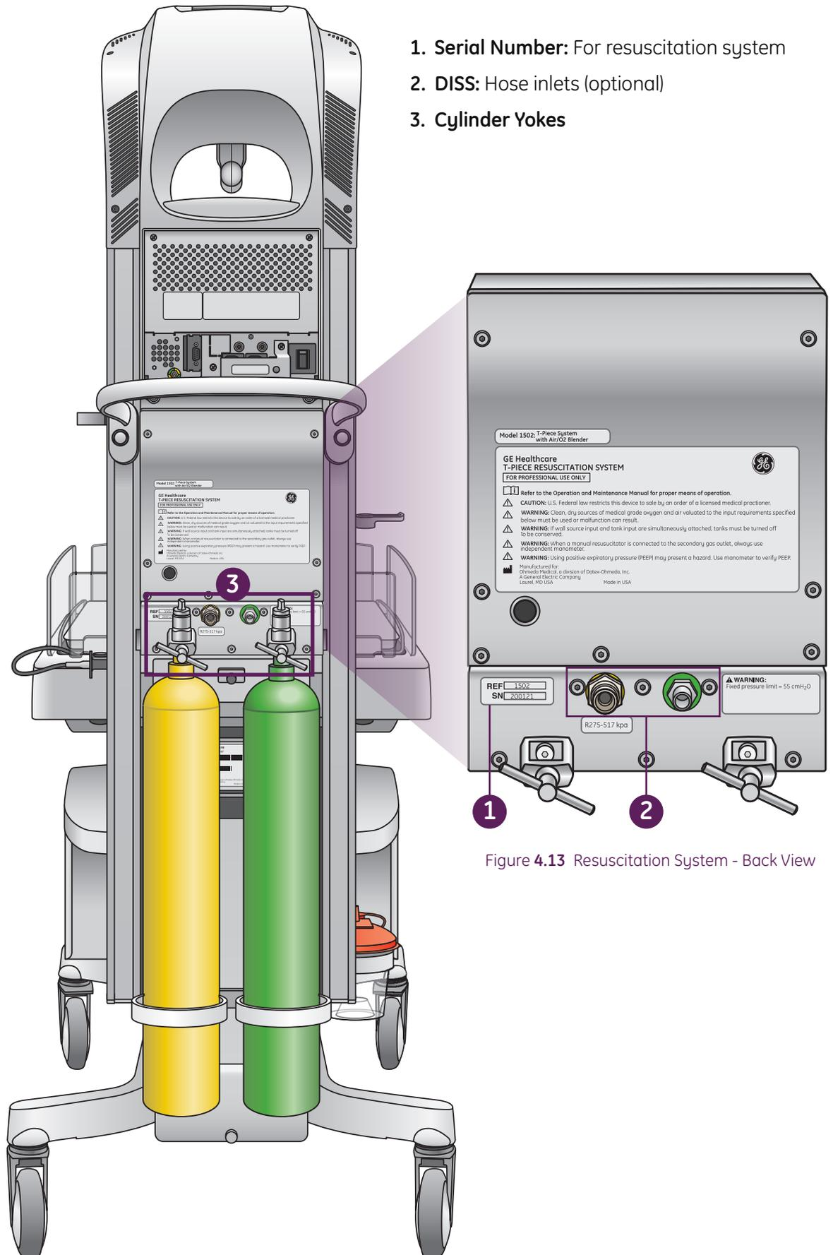
Figure 4.13 Resuscitation System - Back View
