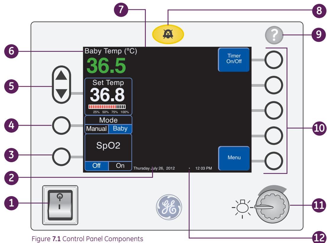
Figure 7.1 Control Panel Components
