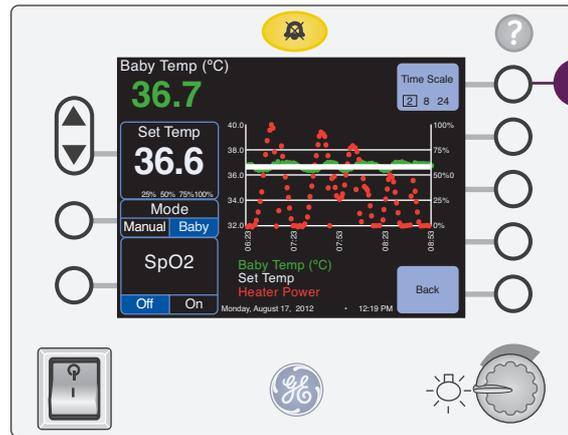
Figure 7.17 Two-Hour Temperature Trend
