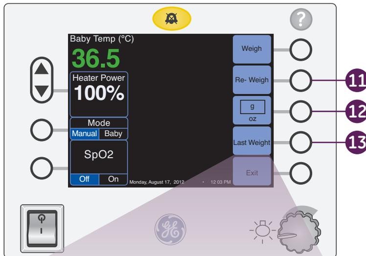
11. Push the **Reweight** key within five minutes of the last weighing sequence if the weight is in doubt. The scale will reweigh the patient without your having to lift the patient to zero the scale.
