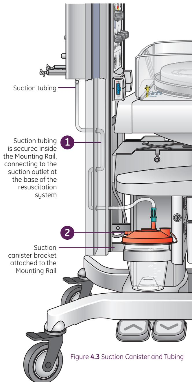
Figure 4.3 Suction Canister and Tubing
