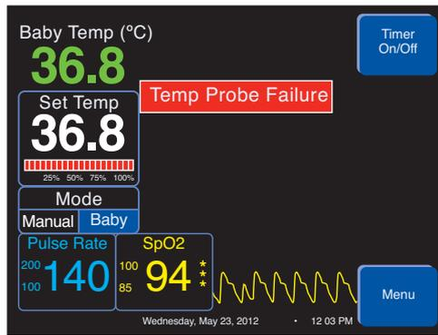
Figure 7.30 Temp Probe Failure Alarm Message
