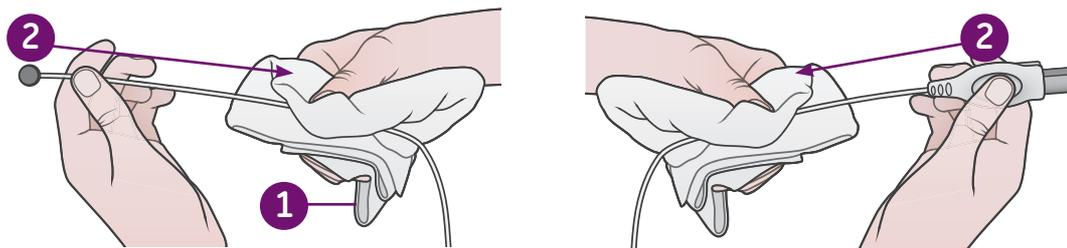
Figure 9.5 Correct Cleaning Skin Temperature Probe Method
