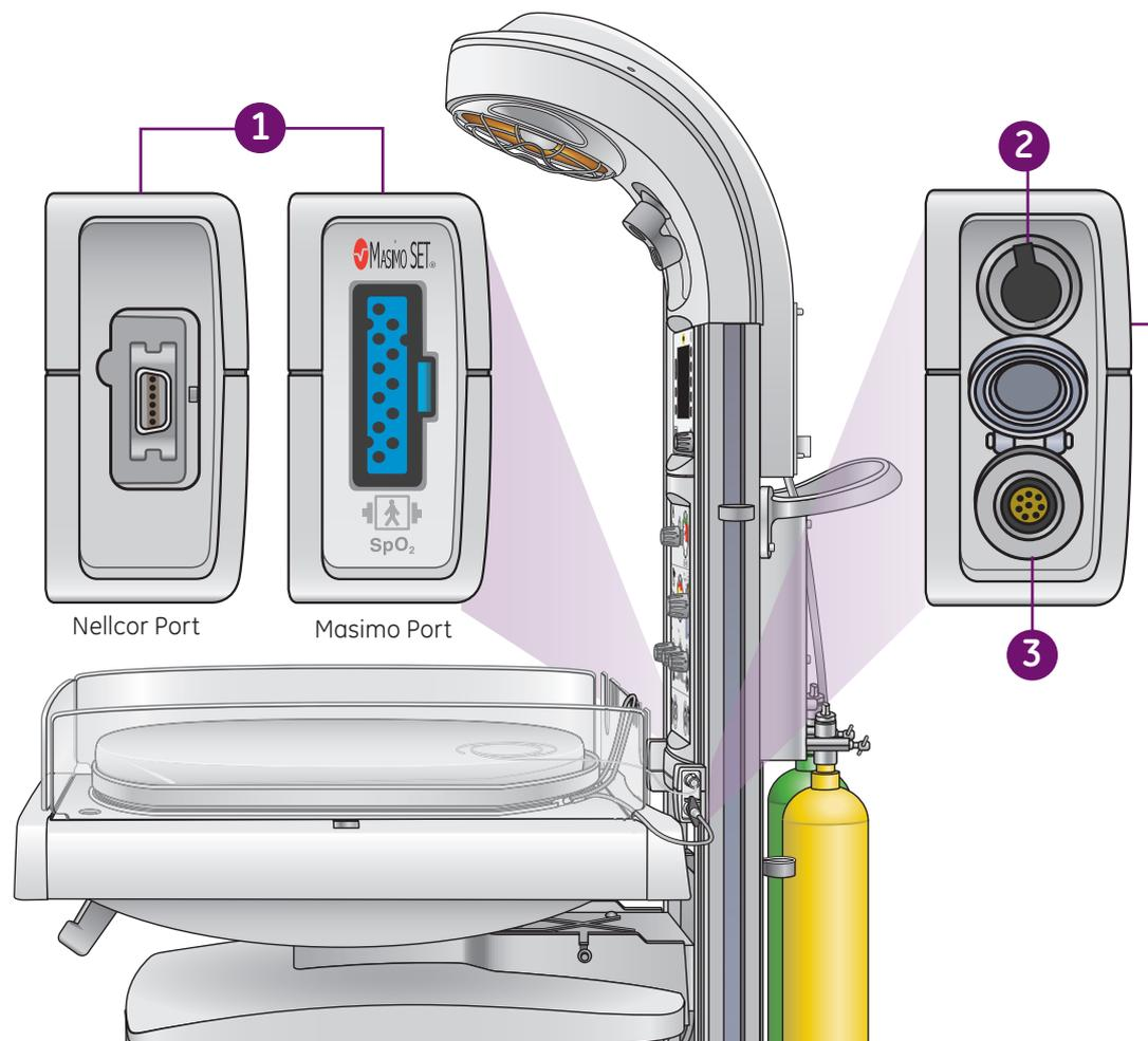
Figure 5.1 Probe Panel Components
