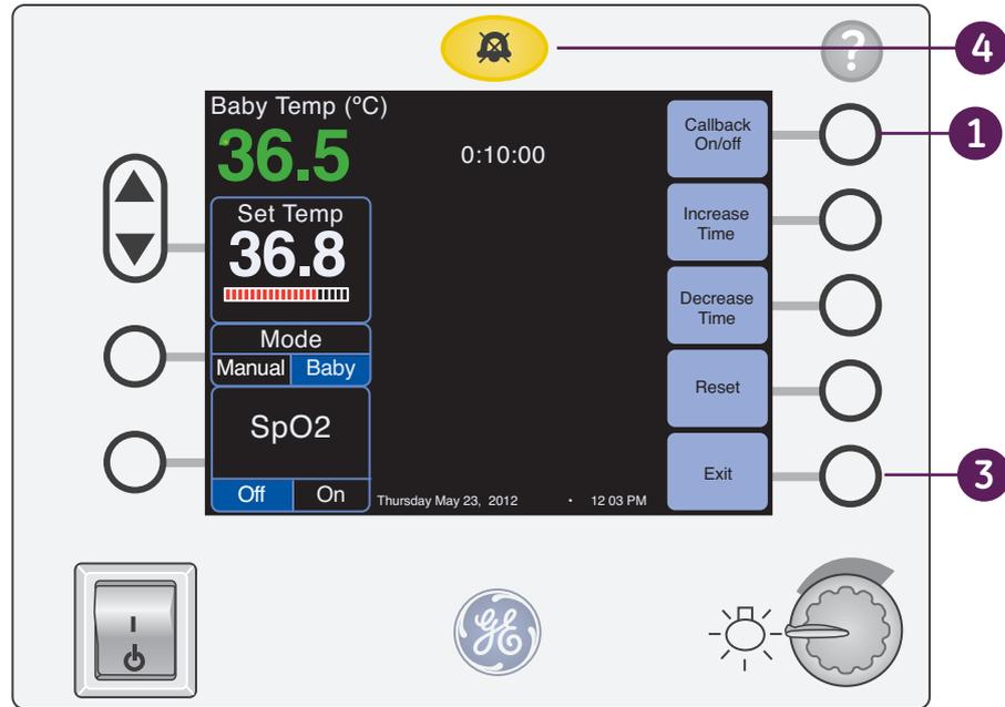
Figure 7.5 Timer ON/OFF Key
