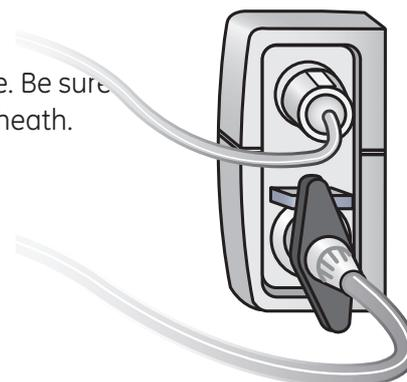
Figure 9.3 Correct probe alignment
