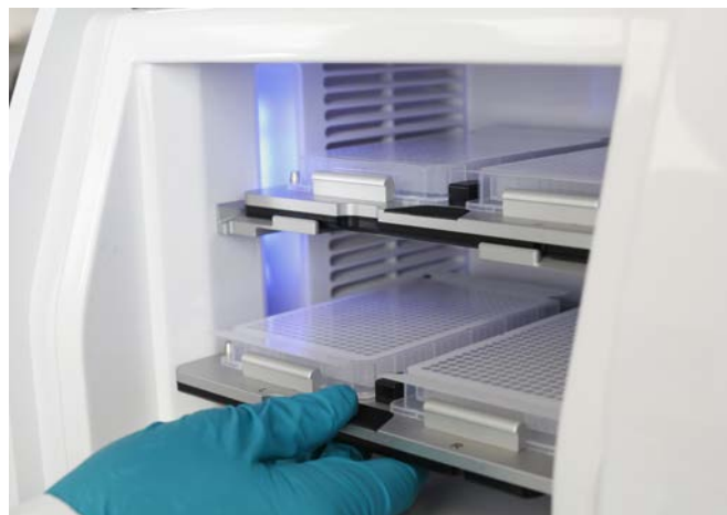
Fig 7. Biacore 8K accommodates up to four 96- and 384-well microplates simultaneously, all in a temperature-controlled environment for optimal assay performance or to ensure sample integrity in extended runs.
